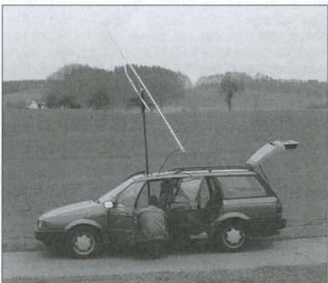
DL3OCH's portable 23cm EME setup
